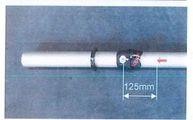
ATTACH THE PLASTIC WASHER OVER THE CENTRE OF THE RIVET HOLE WITH THE STICKY PAD.
