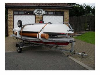
Position the second boat on Upper Cradle section and fit launch trolley on top. Carefully secure the boats ready to travel.
