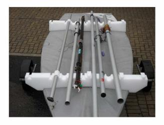
When boat cover is in place, rest the Lower Cradle halves on the fore and aft deck as illustrated above.
