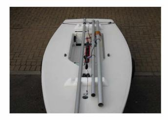
Position the spar carrier on the deck, fore and aft of the boat. Fit spars into place (cord not included).
