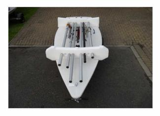
Place the spars appropriately in the slots and fit the Upper Cradle in place, securing the spars between the Cradle halves.
