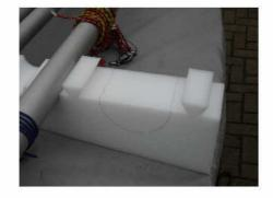
6. Separate cradle and join the semicircles on either side with a straight lines.
