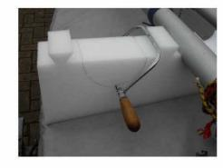
7. Using a 'coping saw' cut out the stencilled semi-circle.
