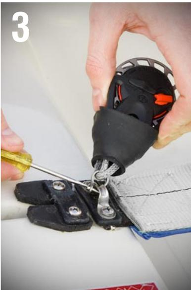
**3** Tighten the shackle with a screwdriver making sure that the shackle is positioned with the pin at the bottom against the saddle (and so the 'bow' portion is over the Dyneema® link).
