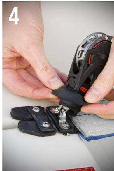
**4** Roll down the boot and align it over the saddle/deck clip.
