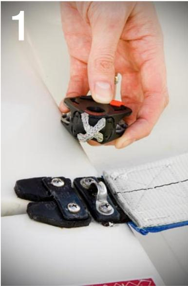
**1** Twist Dyneema® link to form an 'X' and secure in place using the supplied retainer clip.
