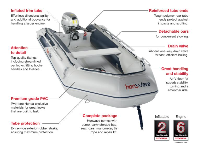
Light and fast, the revolutionary air V-floor inflatable gives rib-like performance that smooths out even the choppiest waters and ensures maximum stability at virtually any speed. The hull design also incorporates inflated rear trim pads, for effortless directional agility and additional stern lift. This has the dual benefit of helping the boat to plane with smaller horsepower engines, as well as providing extra buoyancy for larger engines.
