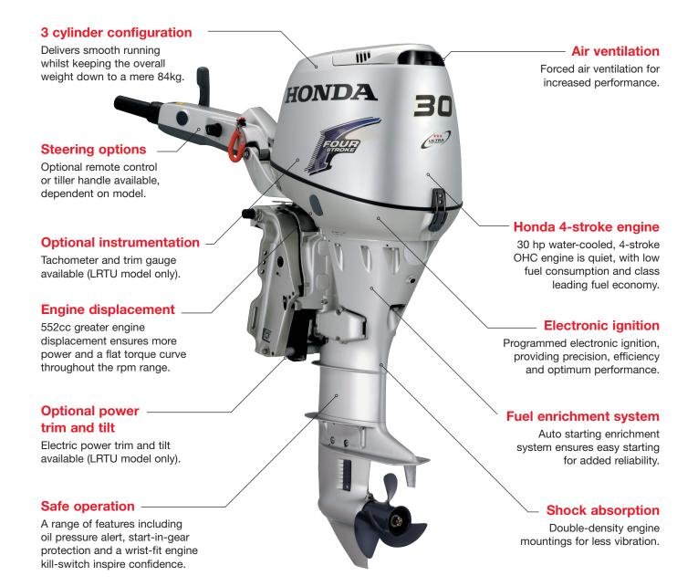
The BF30 is the lightest and most economic 4-stroke engine available in its class, offering smooth and reliable performance. Honda's unique PGM-IG technology provides smoother acceleration, advanced fuel efficiency and improved overall performance.
