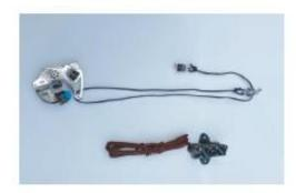
Step 1 - Start by tying a bowline to the top of the double block. Run the line through the block and vang key as per the picture.
