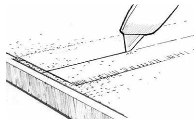
Figure 27 Trim overlapped cloth after the epoxy gels.
