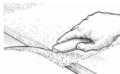
Figure 26 Trim excess cloth after the epoxy gels.
