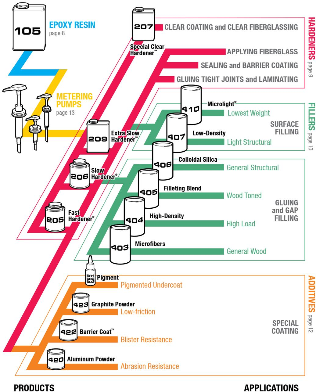
**1** Start with 105 Epoxy Resin, the basic ingredient of all WEST SYSTEM Epoxy compounds. Use 300 Mini Pumps for convenient and accurate metering.
