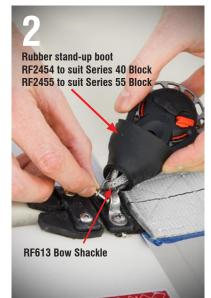
Slide the inverted rubber stand-up boot over the loop and slide it up the block as far as possible.
