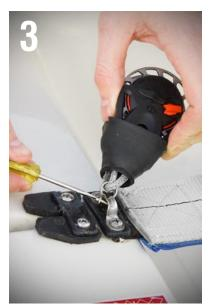
Tighten the shackle with a screwdriver making sure that the shackle is positioned with the pin at the bottom against the saddle (and so the 'bow' portion is over the Dyneema® link).
