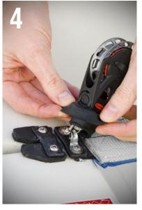
Roll down the boot and align it over the saddle/deck clip.
