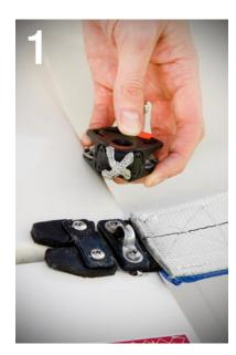
Twist Dyneema® link to form an 'X' and secure in place using the supplied retainer clip.
