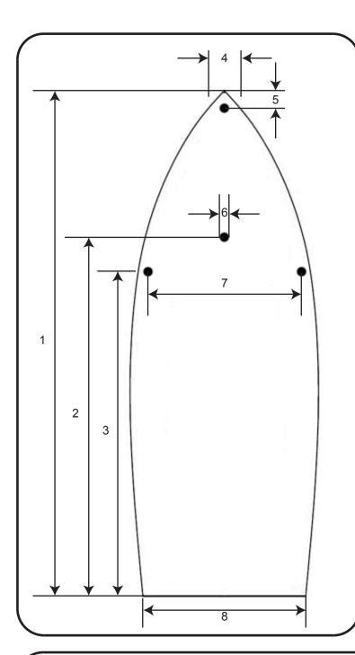
1. Overall Length 2. Transom to back of Mast 3. Transom to Shroud 4. Bow Width 5. Bow to Forestay 6. Mast Diameter 7. Shroud to Shroud 8. Transom Width -
