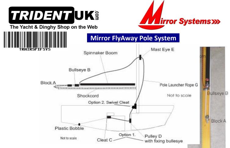
**Block A**. Fit to top of boom, slightly off centre to starboard 610mm from aft end of boom, pulley nearest to mast.
